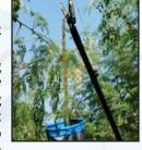
hold the drumstick pod in the collecting bag first and then detaching the pod from the tree by cutting blades operated by the lever. The detached pod is collected in the collector bag.
