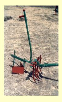
10. Sugarcane trash shredder for 90 cm row spacing
