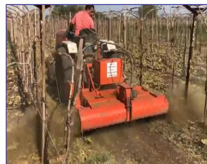
**2. Phule Hydro-Mechanically Controlled Offset Orchard Manager** - Tractor operated Phule Hydro-Mechanically controlled offset orchard manager is recommended to release for old root cutting and bed breaking operations simultaneously in orchards.
